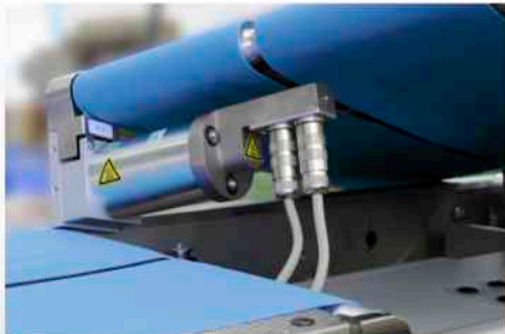
All conveyor connectors are water protected according to IP 67.
