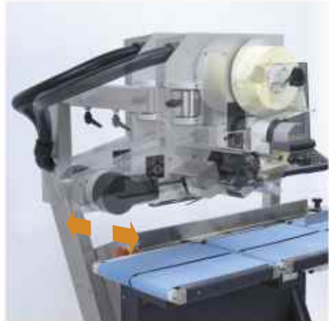
Label placement by lateral printer adjustment
