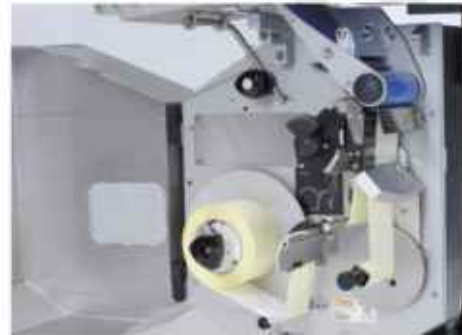
Bottom printer with a label roll of up to 210 mm and a splashproof housing
