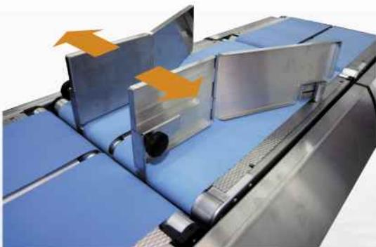
Automatic adjustment of alignment station.
